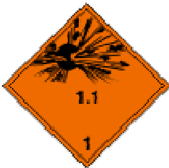
Class 1 Hazard Division 1 Symbol (UN Hazard Division 1 corresponds to MSER hazard type 1)
